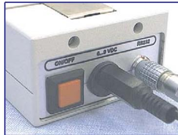
*Fig. 5.4. AC/DC adaptor connection*
