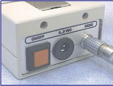
*Fig. 5.3. RS-232 interface cable connection*
